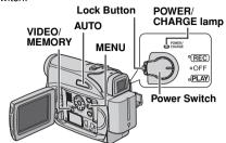
Choose the appropriate operation mode according to your preference using the Power Switch and **VIDEO/MEMORY** Switch.
